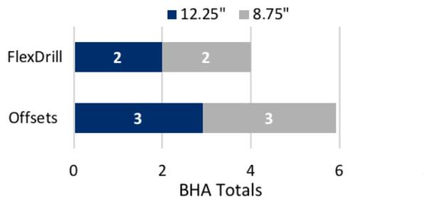
The proper bit engagement and reduced downhole vibration achieved by FlexDrill makes it the obvious leader in BHA efficiency, demonstrated by fewer BHA totals in both the intermediate and lateral sections.
