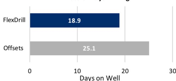
FlexDrill ROP efficiencies contributed to a significant reduction in total days on well when compared with offsets in both the intermediate and lateral sections.
