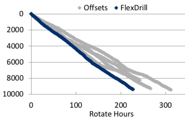
The two depth vs. time charts displayed above compare the rotating performance of the FlexDrill well in the intermediate (left) and lateral (right) sections with their relative offsets. The FlexDrill well, displayed in blue, demonstrates far better performance when compared to the average of the offsets.
